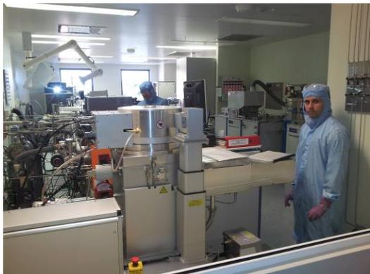
Sentech SI 500D Inductively Coupled Plasma Enhanced Chemical Vapour Deposition (ICPECVD) tool in full swing at the ANFF-WA fabrication facility. The tool is operated by postgraduate student Rohit Sharda.
