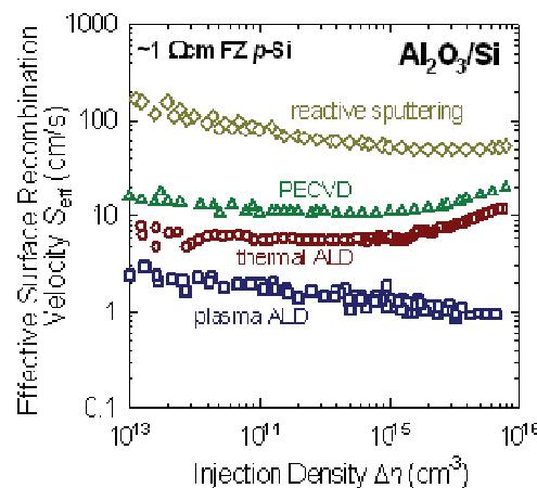
Figure 2: Surface recombination velocity of the reactive sputtering in comparison to other dielectrics.
