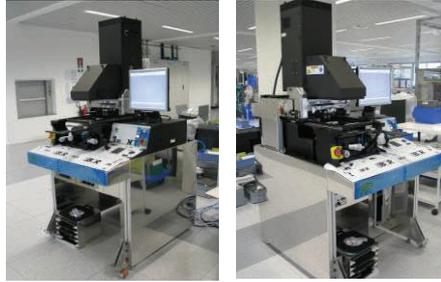
*The new Nano-Imprint Lithography/Hot Embossing system undergoing inspection prior to shipment to ANU*
