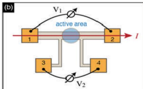
area. A four contact bar structure device (see Fig. 2b, above) was fabricated to measure voltage between two points while applying constant current along the bar as function of pH. These measurements revealed a bath-tub like dependence of sheet resistance with pH, indicating that the sheet resistance increased as a function of ionic concentration, regardless of whether the pH was acidic or basic, and showing that the uncapped AlGaIn/GaN heterostructures are demonstrating selectivity towards
