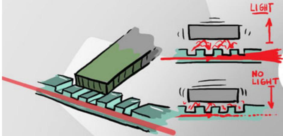
By fabricating a similar nanostructure underneath our beam, and aiming a laser through it, the amount of light that reaches the other side will depend on the height of the mechanical beam.
