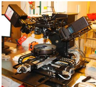
The ACT Node has recently taken delivery and commissioned a new piece of kit in our EBL Laboratory - a Spectral Ellipsometer.
