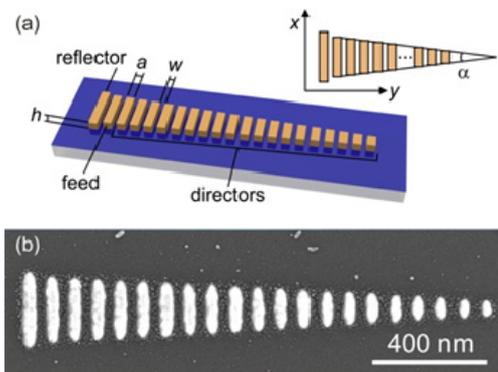
Fig. 1: (a) Design sketch and (b) scanning electron micrograph of a tapered Yagi-Uda nanoantenna for broadband unidirectional emission enhancement [1]
