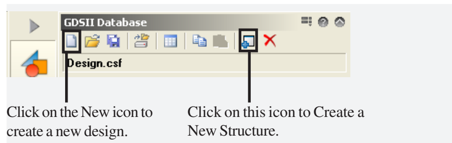
Figure 5-21 Creating a new structure in GDSII Database.
