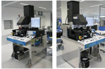
The new Nano-Imprint Lithography/Hot Embossing system undergoing inspection prior to shipment to ANU
